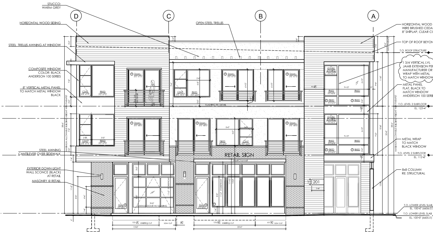
WEST / BROADWAY BUILDING ELEVATION
